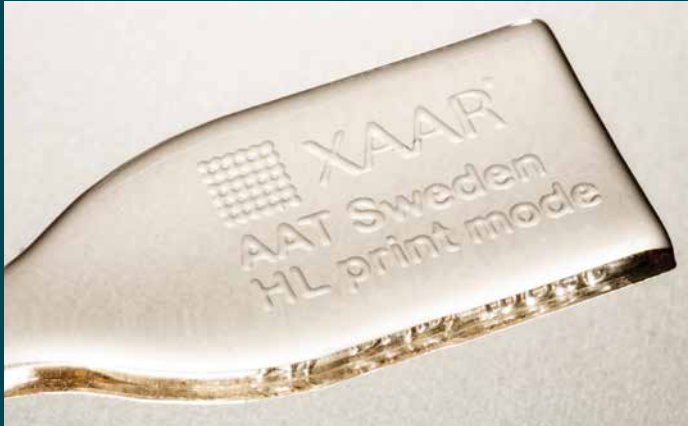
3D printed tensile test bar, produced with BASF photopolymer using a Xaar 1003 GS12 printhead with Xaar's binary jetting High Laydown technology (similar samples were also produced with three-cycle jetting modes also)
