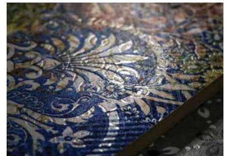
Ceramic tile gloss effect printed by Scientifica Tiles LLP, India at 60 g/m 2 at 24 m/min with Xaar 2001+ GS12 printheads using Xaar's High Laydown Technology
