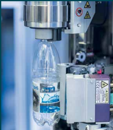
Bottle printing station in KHS printer including UV curing lamp and Xaar 1001 (left image) in 'skyscraper' mode; jetting station with white + four colour direct label printing on bottles (above image)
