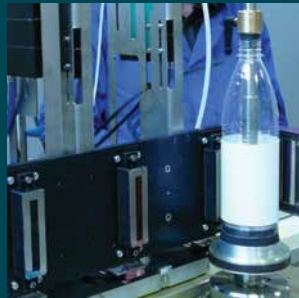
Bottle printing station in KHS printer including UV curing lamp and Xaar 1001 (left image) in 'skyscraper' mode; jetting station with white + four colour direct label printing on bottles (above image)
