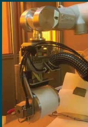
A Xaar jetting test rig with a Staubli robot arm (at the Iprint Institute for Printing, Switzerland) is shown on the left with the close-up on the right showing a Xaar 1003 printhead mounted on the robot arm for jetting at high levels of acceleration and deceleration 11
